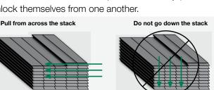
TIP: When taking planks from the pallet installation, avoid repeating the texture pattern by working across the pallet. Two to four planks can be removed from a stack at one time. But then material should be taken from adjacent stacks, again working across the pallet. Texture repeat is typically a concern on large walls with few breaks such as windows or doors.
