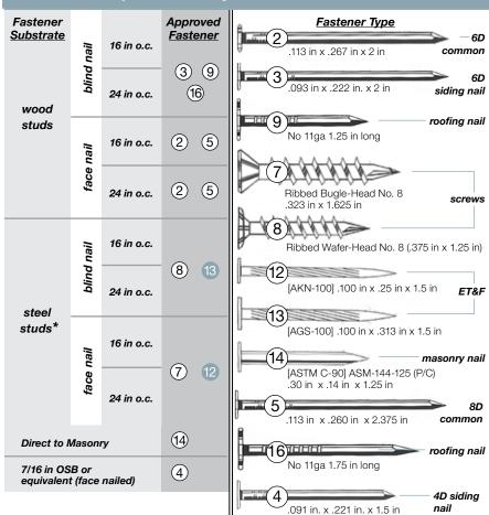
\*When blind fastening 9.5 in or wider product onto steel studs, use screws.
