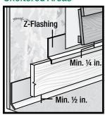
Figure 11 Mortar/Masonry
