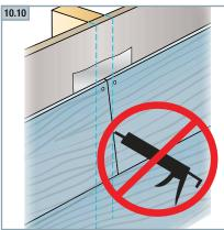
Caulking at HardiePlank lap siding butt joints is not recommended for ColorPlus for aesthetic reasons as the caulking and ColorPlus will weather differently. For the same reason, do not caulk exposed nail heads. Refer to the ColorPlus touch-up section for details
