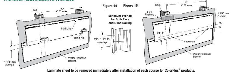
Pin-backed corners may be done for aesthetic purposes only. Finish nails are recommended for pin-backs. Headed siding nails are allowed. Place pin-backs no closer than 1 in. from plank ends and 3/4 in. from plank edge into min. 3/8 in. wood structural panel. Pin-backs are not a substitute for blind or face nailing.
