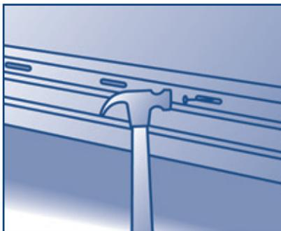
2. Install the back skirting trim. Snap a chalk line at the bottom of your home to mark the position for the back skirting trim. Nail the trim pieces to the home using the nail slots. Make sure you place the nail in the center of the slot and do not hammer tightly.
