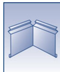
6. b) Cutting inside corner. To cut the front skirting trim for inside corners, cut out a 1" or 2" tab in the top edge of the spring lock and make a small "V" cut through the bottom lip. Bend and snap the trim piece into place.
