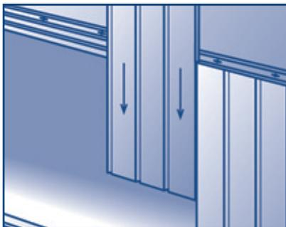
4. Measure the skirting panels to the proper height, subtracting 1/4" for expansion. Cut the panels to size, using tin snips. Slide panels over the back skirting trim and into the vinyl ground channel, interlocking the panels as you install them. To form corners, bend but do not cut the panels.
