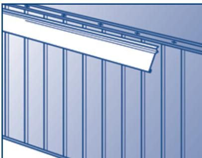
5. Snap the front skirting trim into place to hold panels securely. To form corners, do not cut the panels, notch and bend the panels. Follow the special guidelines shown in illustrations 6a and 6b to finish the skirting trim at the corners.
