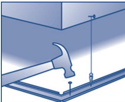
1. Install the vinyl ground channel directly under the outside edge of your home, using galvanized nails. Use a plumb bob to determine exact location.
