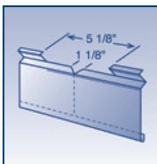
6. a) Cutting outside corners. Determine the location of the corner and cut a 5 1/8" section from the top edge of the spring lock. In the center, cut a "V" 3/4" deep and 1 1/8" wide at the top edge, and a small "V" cut at the bottom. Bend the front skirting trim and snap it into the corner.
