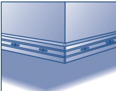
3. To go around corners, bend the back skirting trim at the corners of the home and continue nailing. Do not cut.
