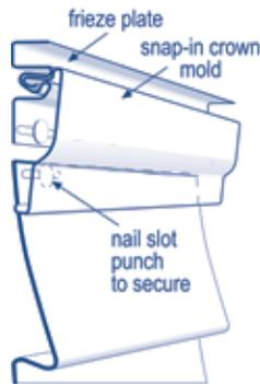
Top panel installation using frieze plate and crown mold
